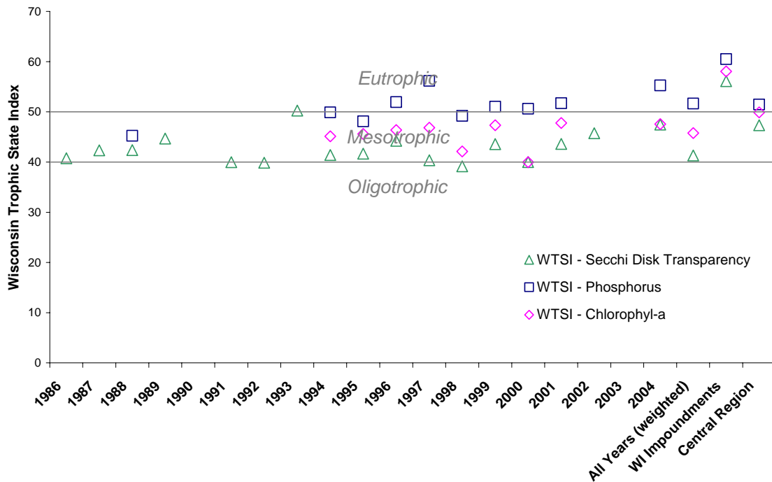
Figure 14. Mount Morris Lake Wisconsin Trophic State Index values for Lake D. Calculated with surface sample data collected during June, July, and August.
