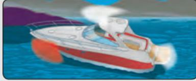
The masthead light and sternlight may be combined as an all-round white light on vessels less than 39.4 feet long.
